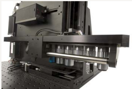
Auto focus system used in LCD manufacture
